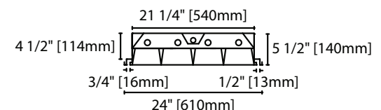
TBDC 2' - 4 Lamps Cross Section View
